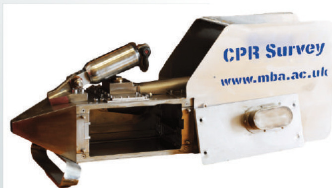
The Continuous Plankton Recorder. Photo: The CPR Survey
